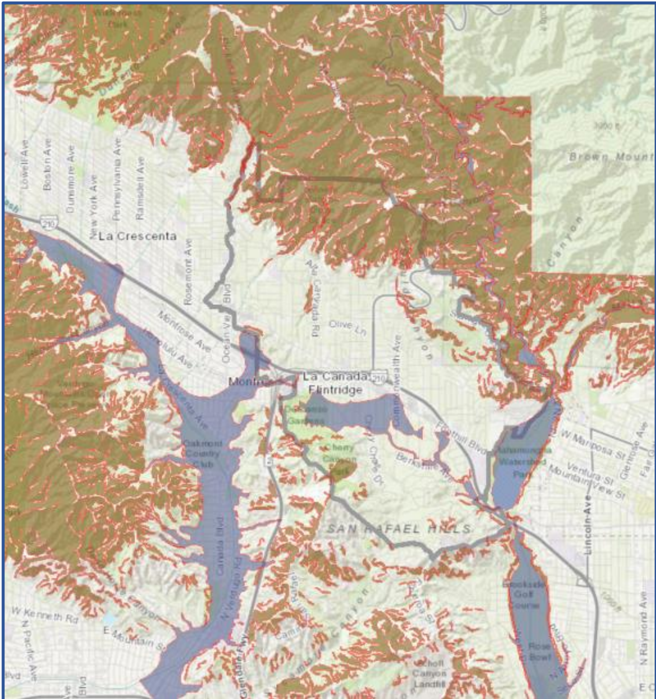
Figure 16: Landslide zones in the City of La Cañada Flintridge. Source, Los Angeles County
